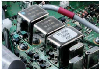
\*For 1.8/3.5/7/14/21 MHz Amateur bands, when receiving in CW/FSK/SSB modes down conversion is selected automatically if the final passband is 2.7 kHz or less.
