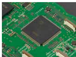
For band scope ADSP-21363 clock @332MHz
