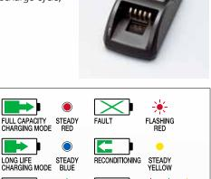
Battery conditions are displayed in color illuminated indicators on the charger, which are also displayed on a connected PC with the same color scheme. Colorcoordinated patterns provide users with at-a-glance information for comprehensive battery management.
